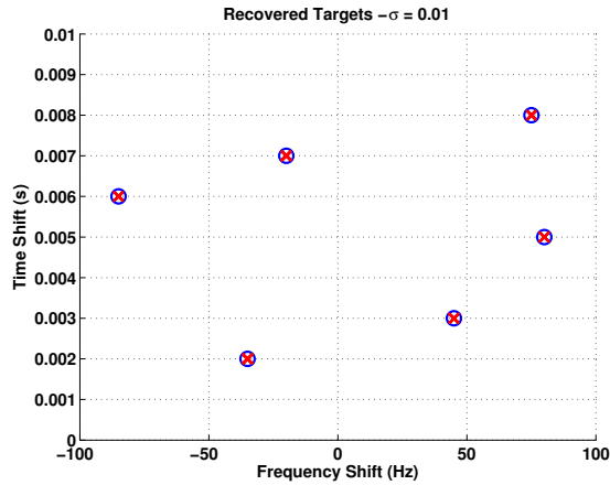
Fig. 7: Estimation of reflector parameters with AWGN \sigma^2 = 0.01 . The true reflector parameters are shown by a blue circle while the recovered parameters are shown by a red x.
