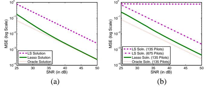
Fig. 2. Numerical results comparing the performance of a lasso estimator with that of a LS estimator. The MSEs of the channel estimates are plotted on a log scale against the SNR in dB corresponding to (a) Spread Spectrum Training Waveforms, and (b) STF Training Waveforms.
